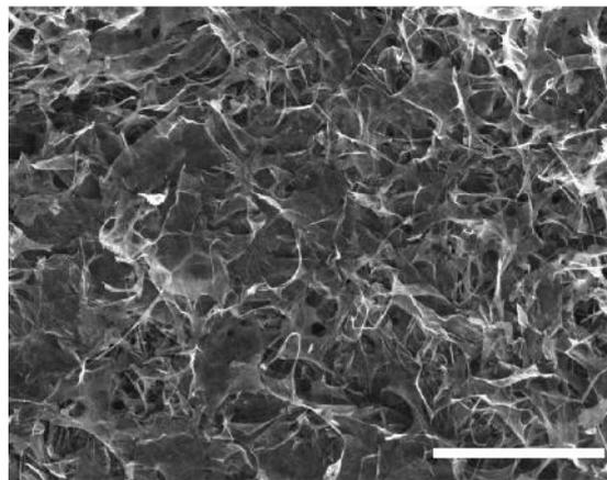
**Figure 1.** SEM images of 3D graphene sponge. The scale bar is 50  $\mu\text{m}$ .
