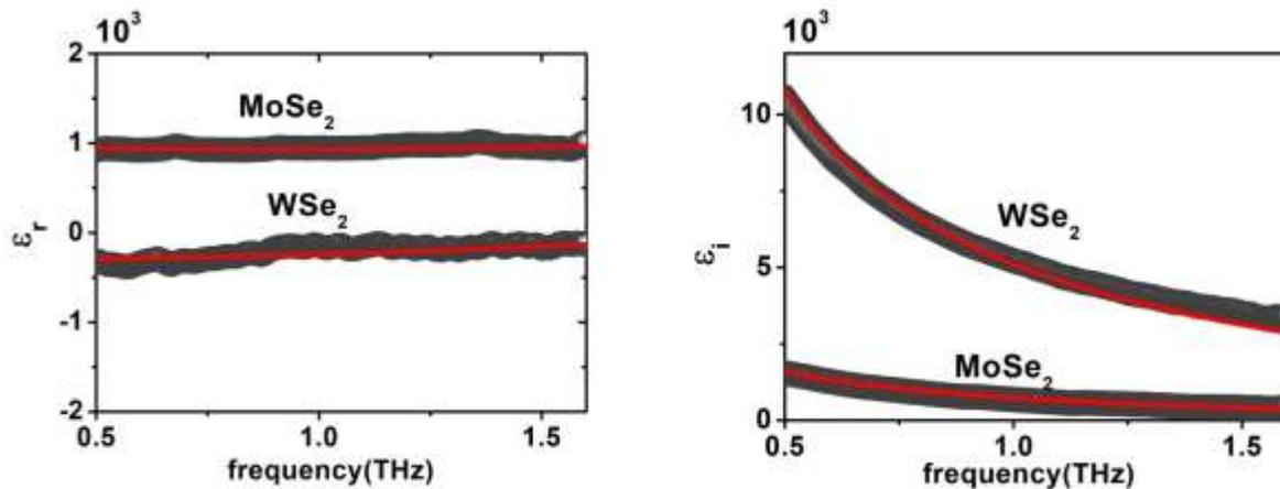
Figure 1: Real (left) and imaginary (right) parts of the dielectric function of measured WSe<sub>2</sub> and MoSe<sub>2</sub> thin films. Grey dotted lines represent the retrieved components whereas the red solid lines represent the fits obtained using the Drude-Smith function.
