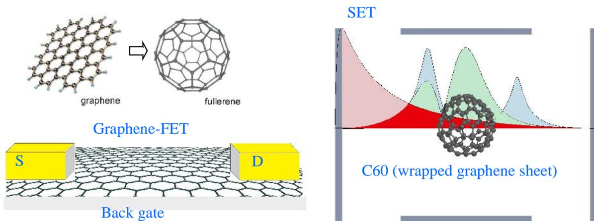
**Figure 1.** Graphene FET and C60 SET. For the latter, we report a sketch the coupling between an atomic cluster and lateral electrodes, through superposition of electronic wavefunctions and effective potentials.
