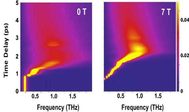
**Figure.** Frequency and time-delay-dependent energy loss function of photo-stimulated  $\text{La}_{1.885}\text{Ba}_{0.115}\text{CuO}_4$ , measured at  $T = 5$  K in absence (left) and in presence (right) of a 7 T magnetic field oriented along the  $c$  axis.
