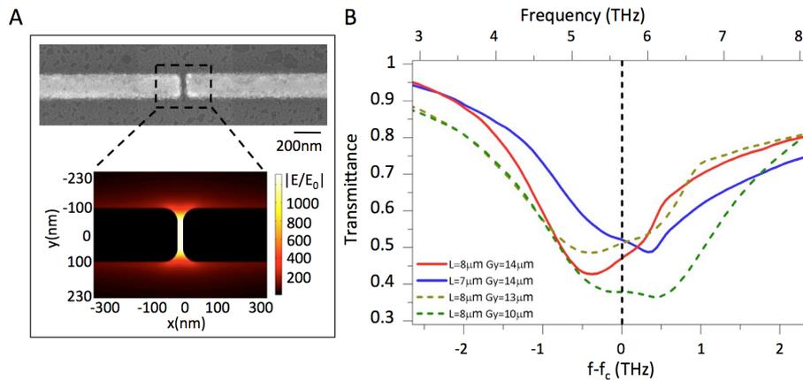
**Figure.** (a) SEM detail of a nanogap region covered with a QD monolayer. The electric field enhancement under resonant conditions is reported in the bottom panel. (b) Normalized transmission of nanoantenna arrays (for different length  $L$  and spacing  $G_y$ ) covered with CdSe QDs.  $f_c$  represents the QD phonon mode frequency.
