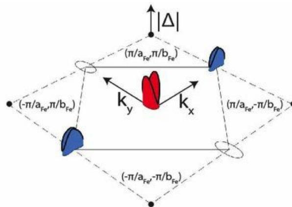
**Figure.** Superconducting gap structure extracted from quasi-particle interference, and modelled quantitatively by orbital selective spin-fluctuation theory. The red/blue “inverted bishop’s hats” illustrate the superconducting gap in momentum space.
