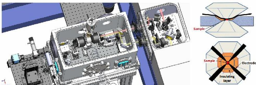
**Figure.** Schematic view of the ultra-high pressure Low Temperature set-up allowing for measurements of the resistivity (left) and diamond anvil cell showing the diamond anvils, the gasket, the sample and the electrodes
